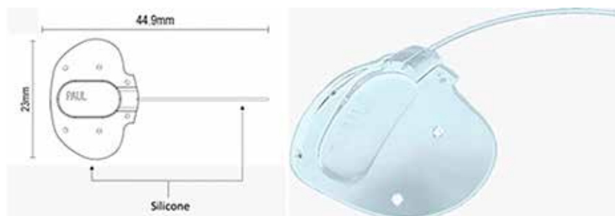
Figure 3. Paul glaucoma implant design (Advanced Ophthalmic Innovations). 13
